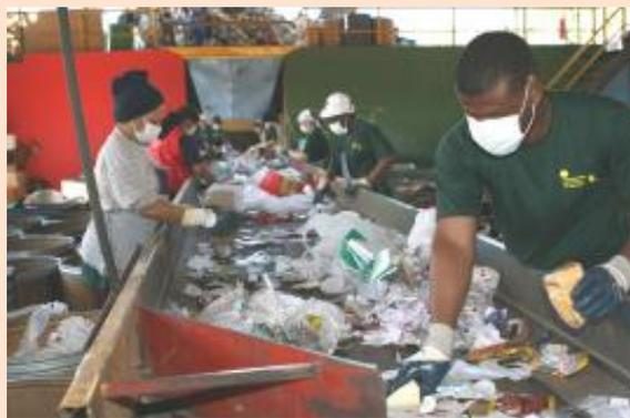
FIGURA 58 – DETALHE DA TRIAGEM DOS MATERIAIS
