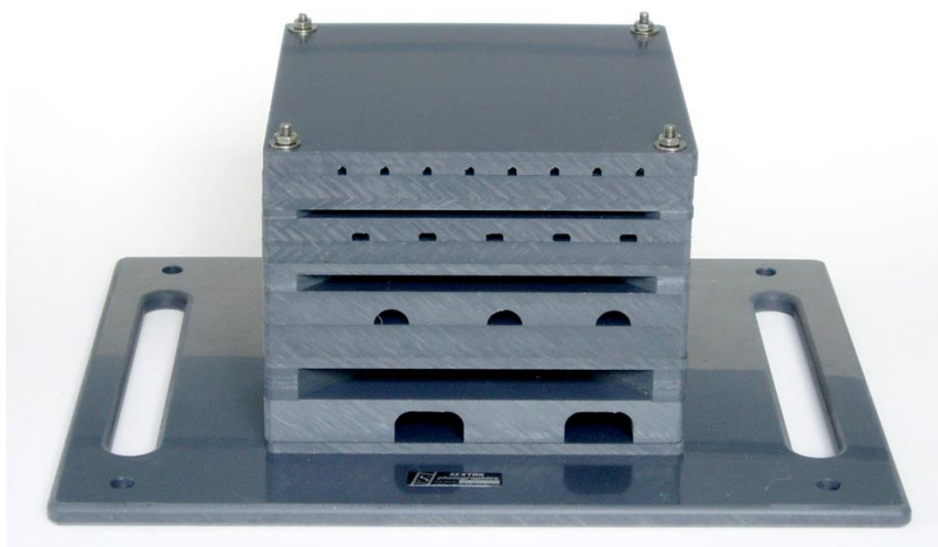
Figura 5 - Modelo do Autonomous Reef Monitoring Structure - ARMS. Fonte: www.pifsc.noaa.gov/cred/survey_methods/arms/overview.php
